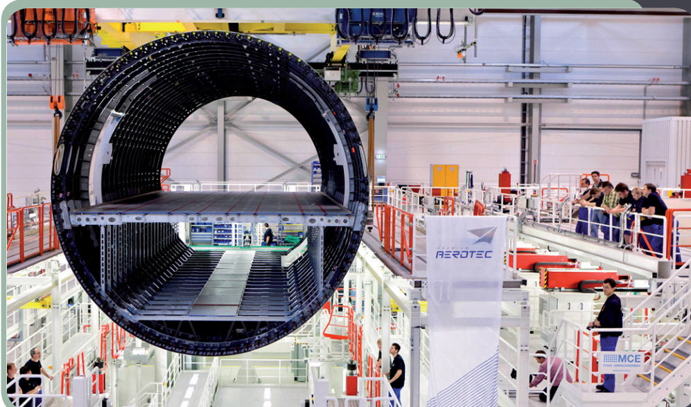
Pictured: Aircraft body parts and structures, produced by Premium Aerotec
